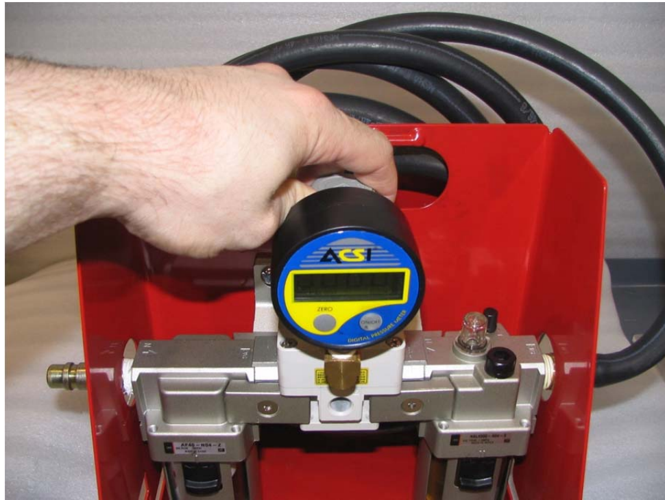
Figure 21. Adjusting FRL Regulator
