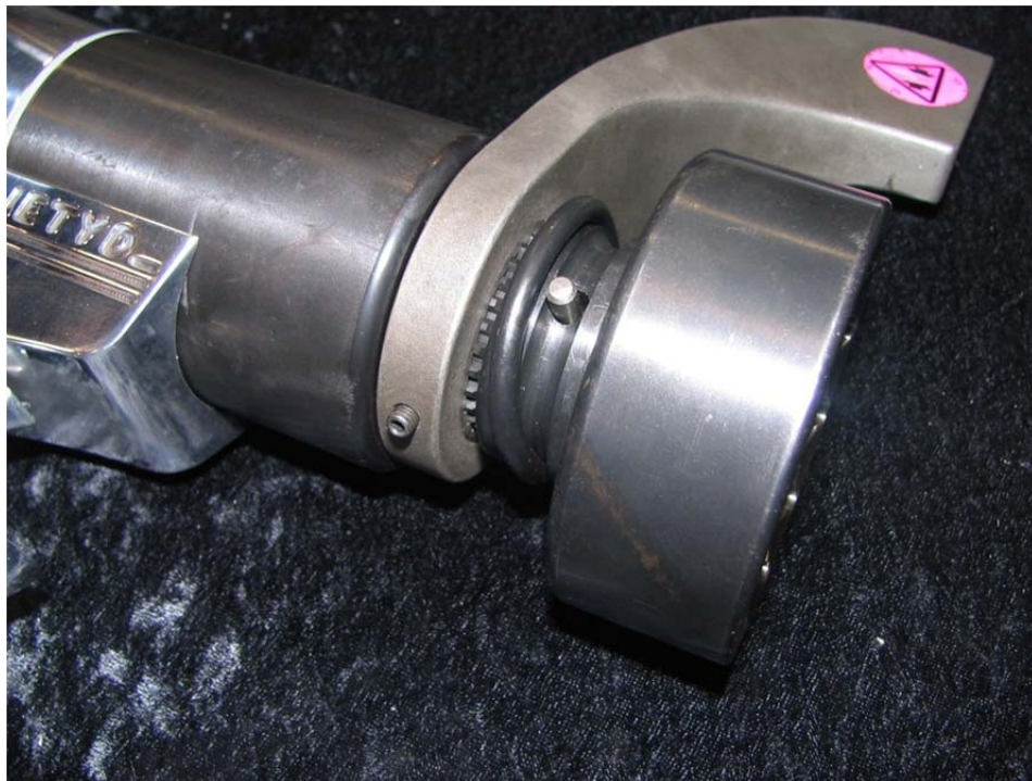
Figure 7. Installing Socket Locking Pin and Retaining Ring
