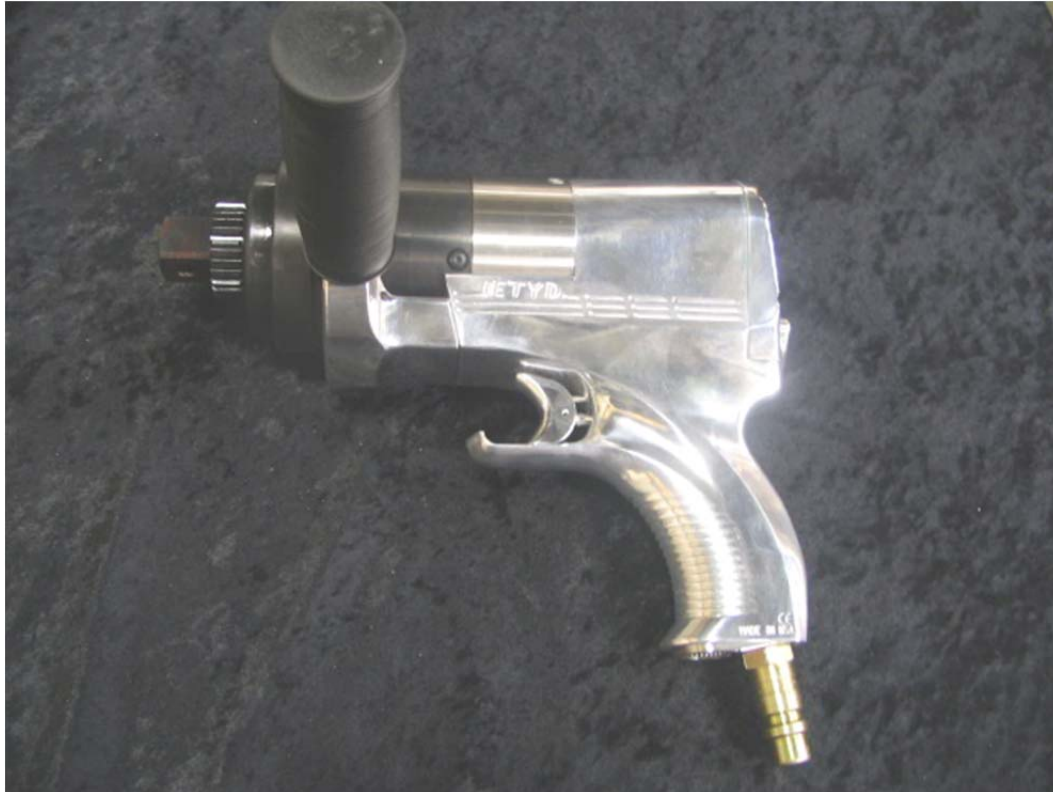
Figure 12. Dual Speed jGun with Handle
