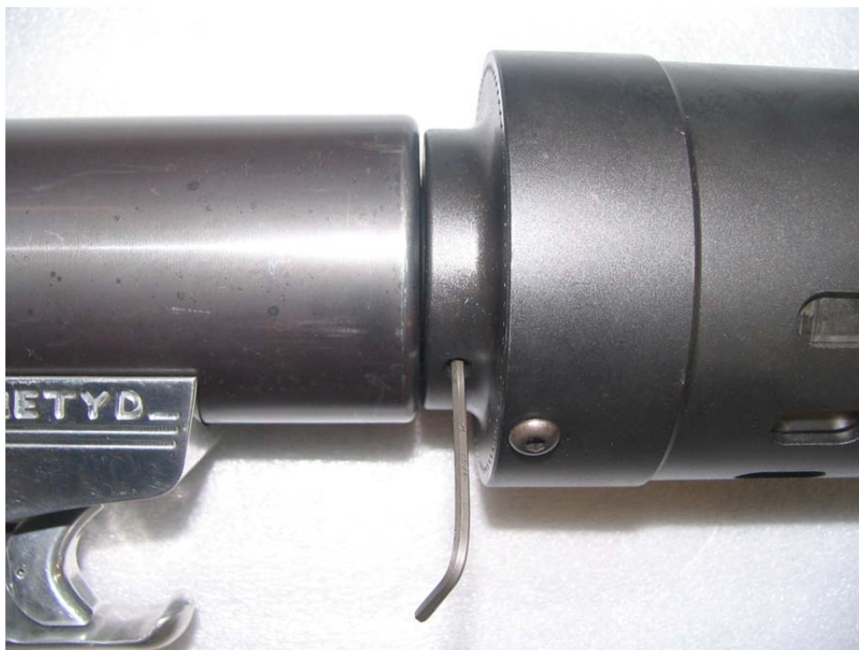
Figure 27. Tightening HYTORC Washer Set Screw
