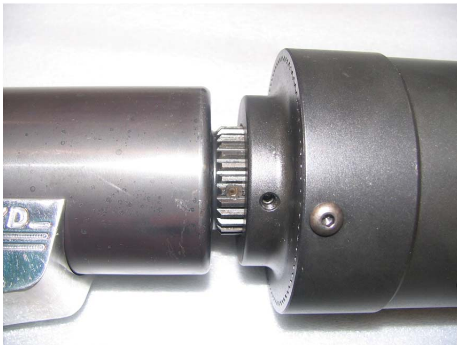
Figure 26. Aligning HYTORC Washer Socket Set Screw with Machined Recess in jGun Splines
