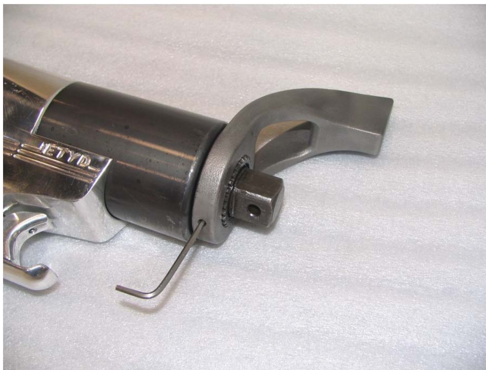
Figure 5. Tightening Reaction Arm Set Screw
