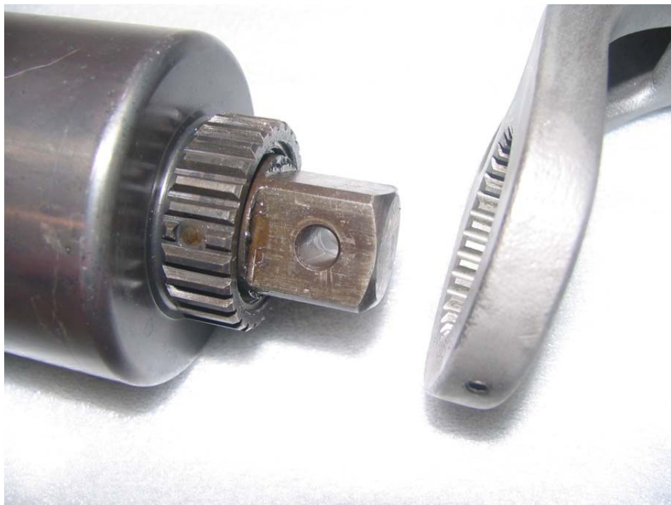
Figure 3. Installing a Reaction Arm
