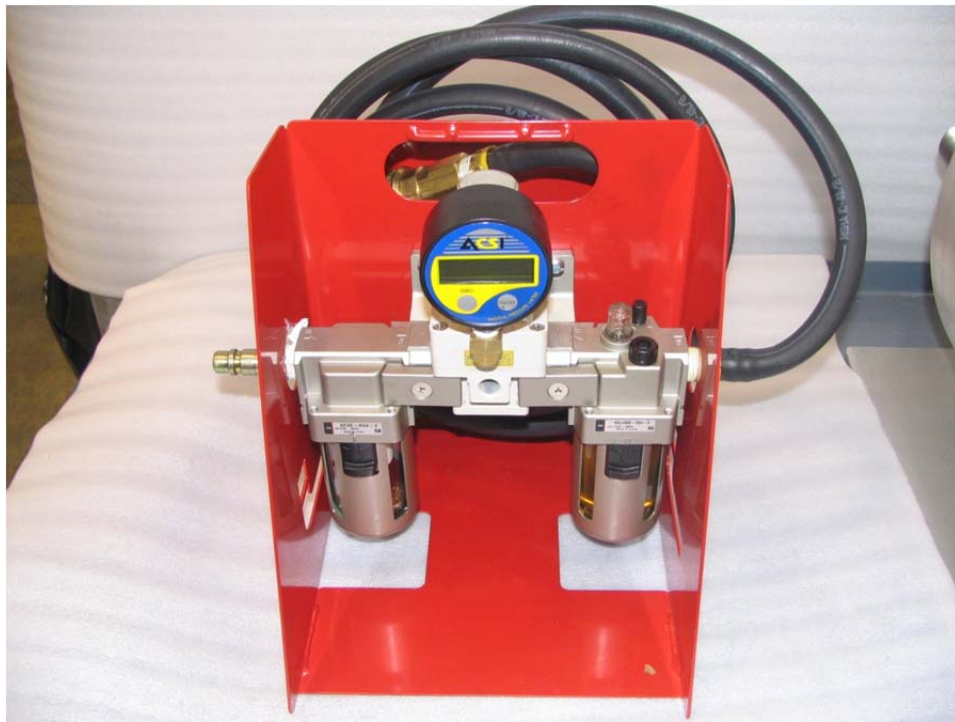
Figure 17. FRL Unit (Shown without silencer)
