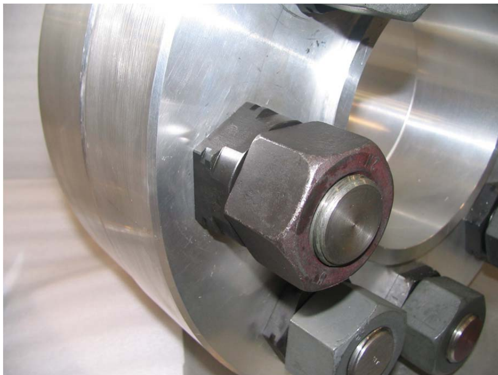
Figure 25. HYTORC Washer Installed
