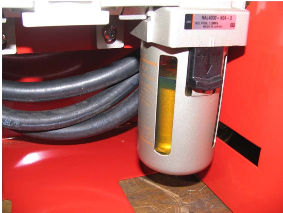
Figure 20. FRL Unit – Lubricator 2/3rds Full of Oil
