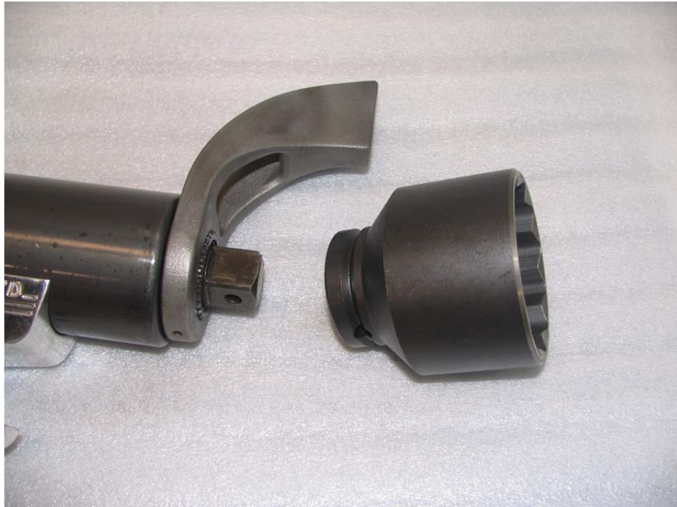
Figure 6. Installing jGun Socket
