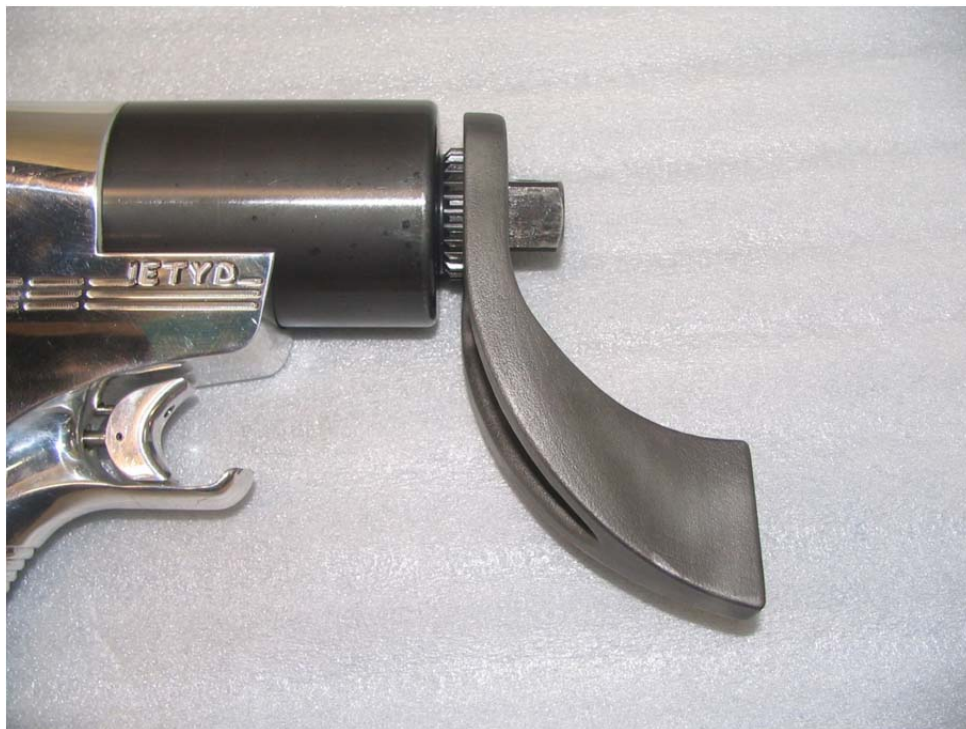
Figure 4. Reaction Arm Installed
