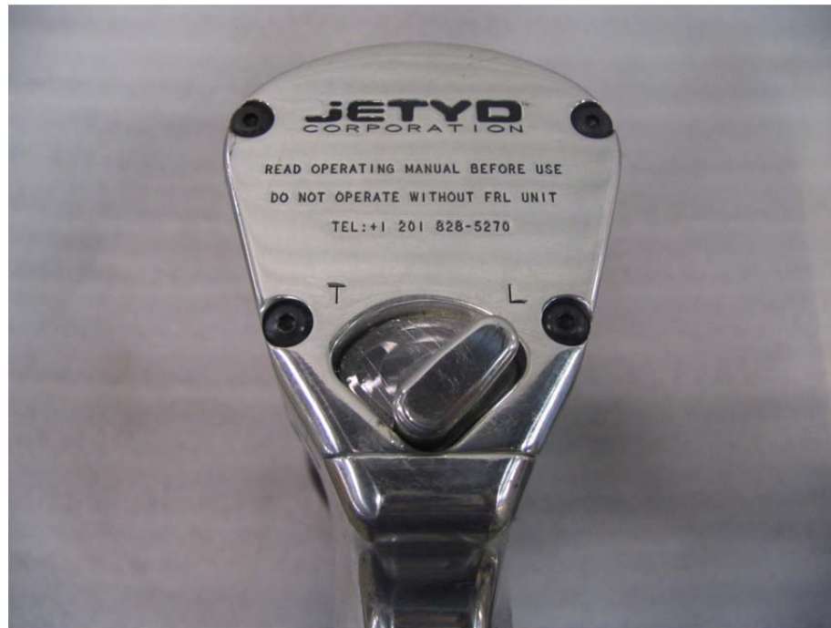
Figure 9. jGun Drive Direction Lever
