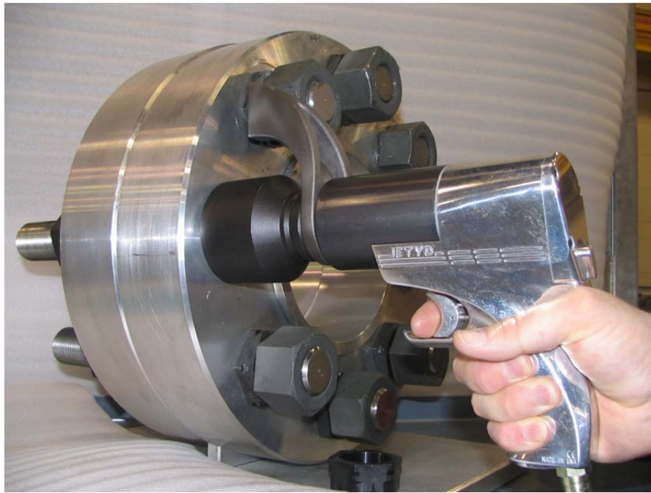
Figure 11. Using the jGun with a Reaction Washer
