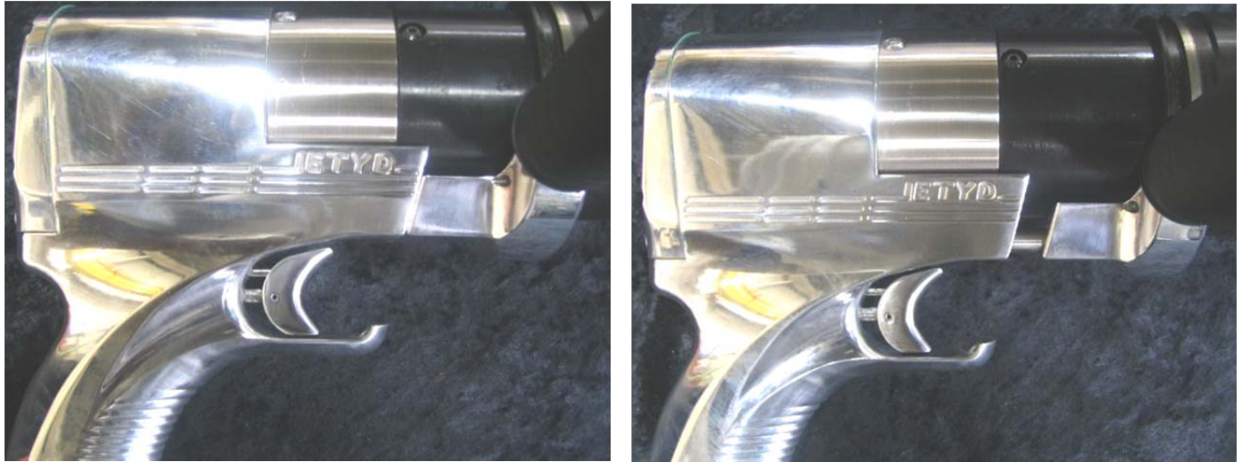
Figure 13. Maximum Torque Setting (Left) and Maximum Speed Setting (Right)
