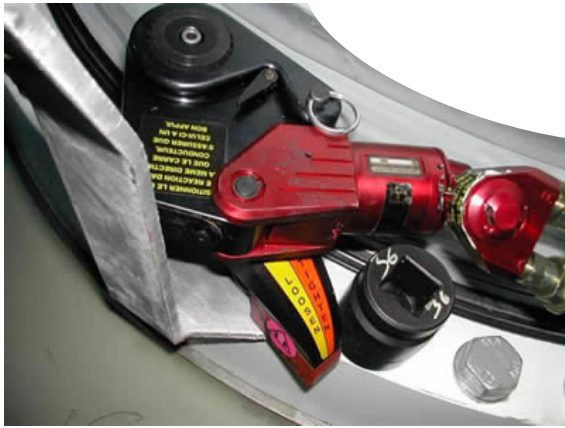
HYTORC-XLCT with the patented square adapter drive system - also deployable with DISC and CLAMP.
