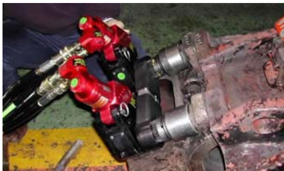
XLCT - TwinTORC without a reaction arm
