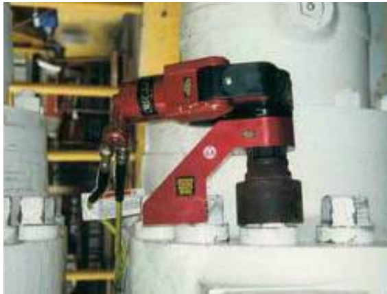
HYTORC-XLCT with the patented square adapter drive system - also deployable with DISC and CLAMP.
