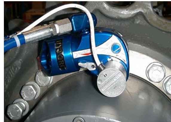
MXT-3 for the assembly of a caterpillar drive, according to the selected rotating angle
