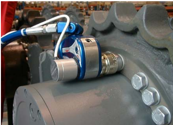
MXT-3 for the assembly of a caterpillar drive, according to the selected rotating angle
