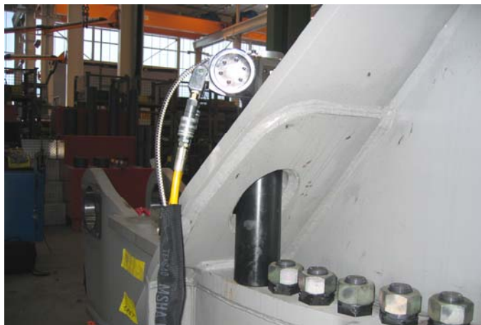
AVANTI-5 with side-load-free axial extension
