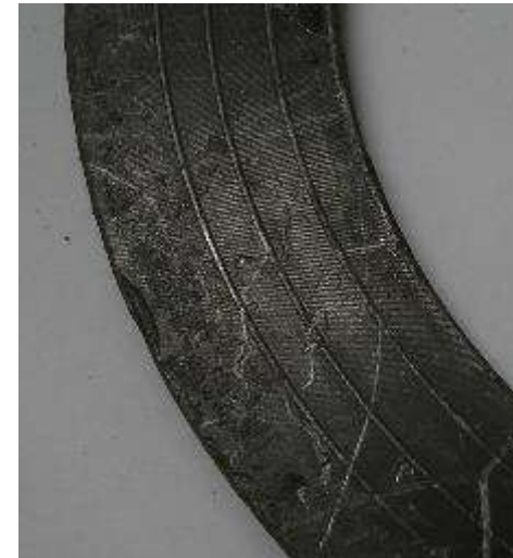
Flange Face Surface Damage
