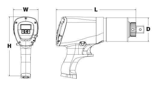
**LEGEND: H** = HEIGHT **W** = WIDTH **L** = LENGTH **D** = OUTER DIAMETER OF GEARBOX
