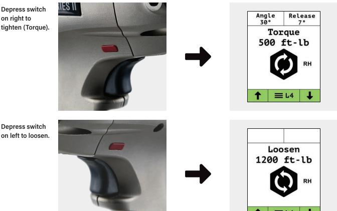
The example shows the change in direction for right hand (RH) fasteners. The directional control switch automatically sets the appropriate direction for left hand fasteners, HYTORC Washers and for the HYTORC Nut as well.
