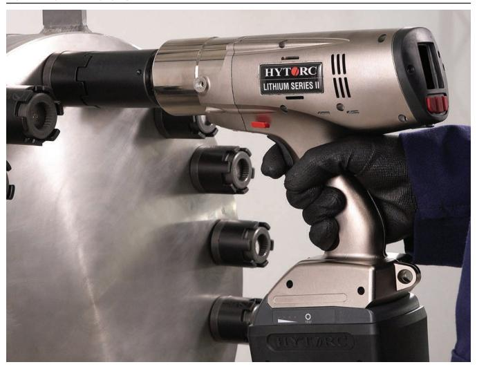
NOTE: The HYTORC Nut inner sleeve is tightened in the counter clockwise direction (left hand threads).
