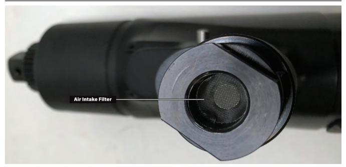
A steady, unobstructed flow of air is critical for proper performance of the **jGun DIGITAL** Tool. The filter in the regulator intake should be cleaned frequently. In heavy use applications this filter may need to be cleaned every day. Apply forced air to unclog and clean the filter for most applications.
