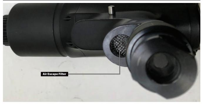
It may also be necessary to clean the larger mesh air escape filters. Inspect and clean filters as needed.
