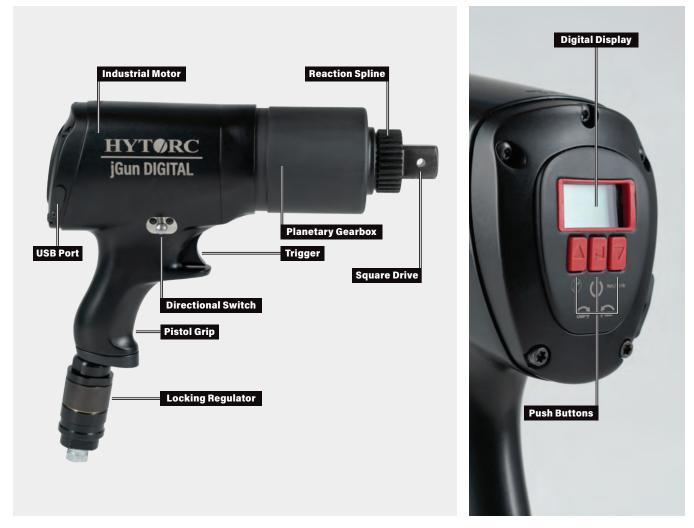
The **jGun DIGITAL** Pneumatic Torque Tool is designed with an industrial grade compressed-air motor allowing the tool to be operated without the need for a separate Filter, Regulator, Lubricator (FRL). High torque is achieved with a rugged planetary gearbox torque multiplier system. The tool is available in a range of sizes with progressively larger drives and gearboxes delivering up to 8,000 ft-lbs of torque.
