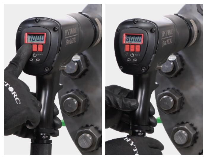
Once the trigger is pulled, the tool freezes the screen and displays the target torque applied. This screen freeze remains in effect until released. To release (un-freeze) the screen press and hold the left button for 3 seconds until the screen flashes once, then adjust the regulator (at least +/- 10% of the previous value). This screen freeze occurs for both tightening and loosening operations.
